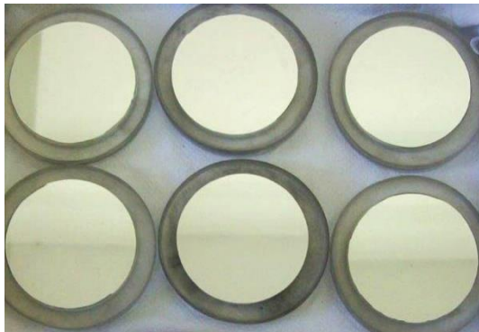
Figure 3. Example of polished surfaces embedded in epoxy resins
